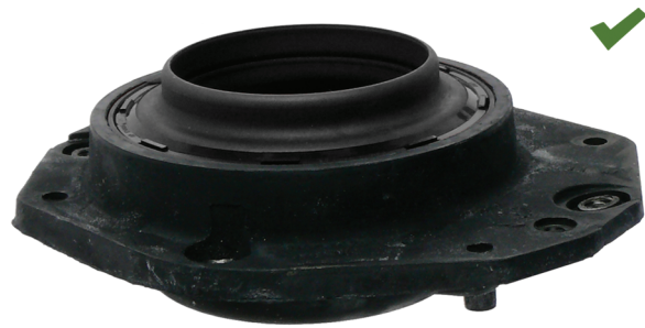
Fig. 2: Suspension strut mount correctly assembled
