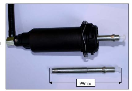
The combined slave and master cylinder fitted to this application is supplied with two pushrods.
