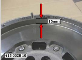
This bulletin is to clarify the catalogue listing for the above vehicles and the compatibility between RepSet and Dual Mass Flywheel. DMF part number 415 0225 10 with RepSet 624 3231 00 is fitted to vehicles built prior to Sep 2006. For vehicles built after October 2006, DMF part number 415 0320 10 and RepSet 624 3267 00 must be used. As not all VRM databases show accurate build dates this may cause compatibility issues if only the RepSet is required.
