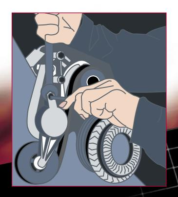
Always check the condition of the automatic tensioner. If it is not functioning properly, replace it with a Gates DriveAlign® tensioner. For more information on Gates DriveAlign® tensioners, please consult leaflet E2/70380 or catalogue E/70378.
