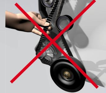
2. Carefully inspect the drive. Poor drive alignment, improper belt tension and worn pulleys all contribute to early belt failure. A complete inspection includes checking for these problems as well as for damage or wear on the old belt. In case of excessive wear replace the pulley immediately.
