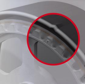
6. Make sure the timing marks are properly aligned, with the engine in Top Dead Centre position. Install the belt, but be careful not to force it over the pulleys. When arrows on the belt are provided, make sure they point in the direction of engine rotation.
