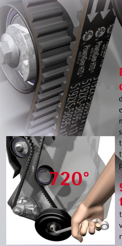
8. Rotate crankshaft (in the direction of normal rotation) exactly 2 complete turns or a multiple of 2, to remove any slack in the belt and to allow the teeth of the belt to seat themselves perfectly in the pulley grooves.
