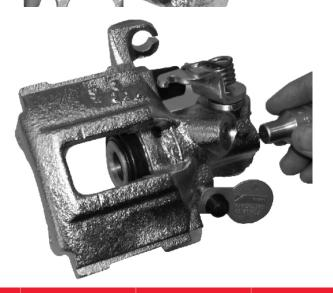
Wind back anti-clockwise until the disc can be turned freely.
