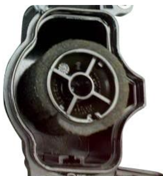
Figure 1: Blocked Filter Element
