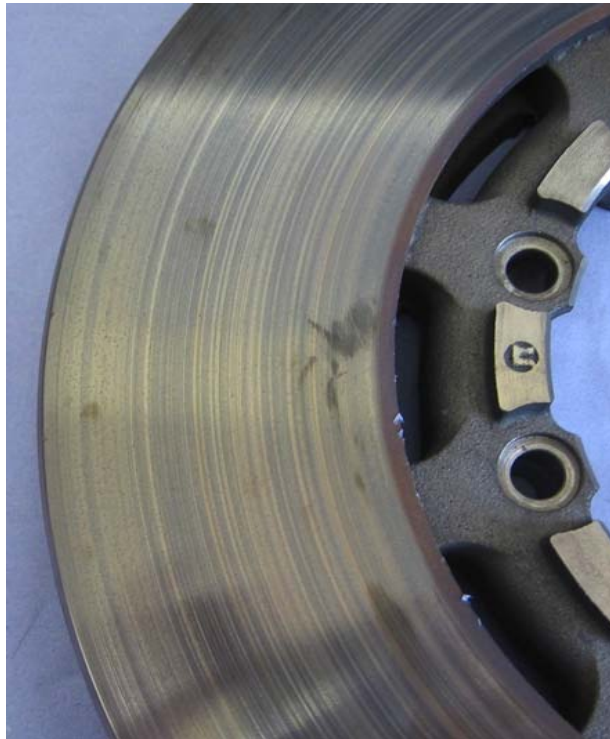
Inboard of Disc After 200 Brake Stops
