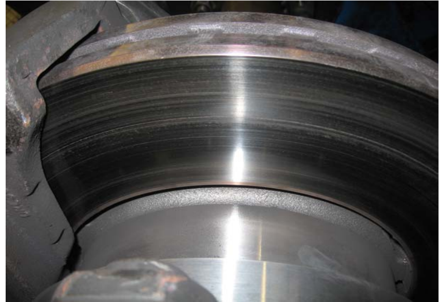
Outboard of Disc After 200 Brake Stops
