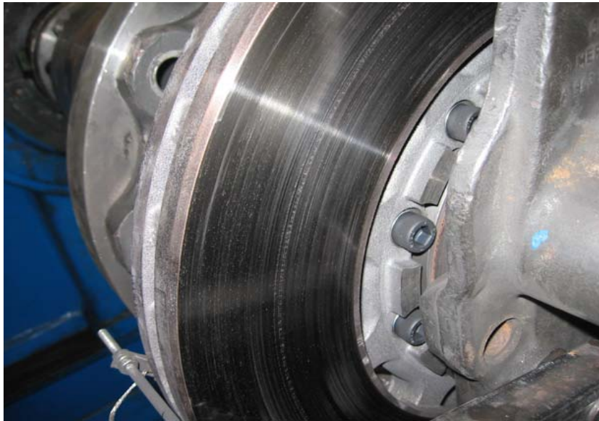
Inboard of Disc After 200 Brake Stops
