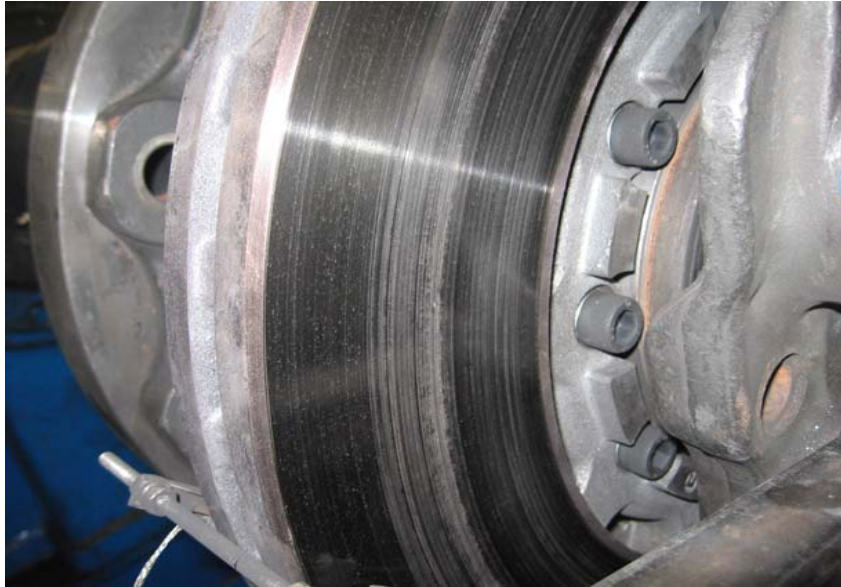
Inboard of Disc After 200 Brake Stops
