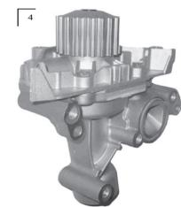
If satisfactory installation is not possible due to distortion of the backhousing replace complete pump (pic 4)
