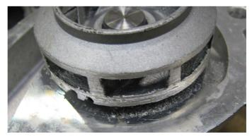
damaged impellor as a result of no locating dowels being fitted!
