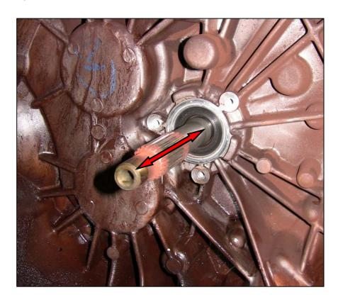
If excessive movement is found then the gearbox must either be overhauled or replaced.
