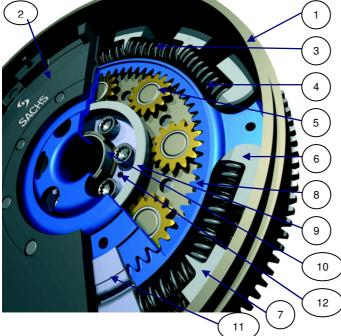
Dual-mass flywheels are installed in many modern vehicles to decrease noise and improve refinement on the move.
