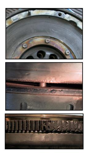
Caused by misuse of the clutch, e.g. clutch slip:
