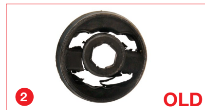
Faulty suspension arm bush
