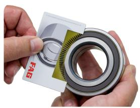
Fig. 1: The encoder card can be used to determine the installation side of a multipole encoder. With passive encoders, this does not work.
