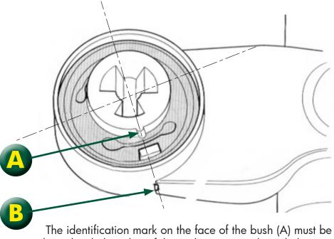
aligned with the edge of the trailing arm on the axle beam (B)
