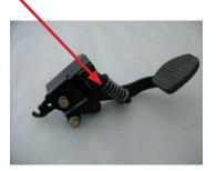
8. The Auto-adjust clutch mechanism can now be released by removing white retention cap - DO NOT REMOVE the white plastic retaining cap until you are sure the Auto-Adjust mechanism is in the correct position, the pedal and gearbox ends of the cable have been fitted correctly and that the cable routing is correct.
