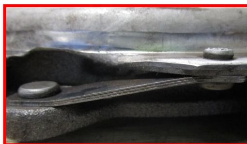
Fitted part returned as warranty; shows deformation/damage to the drive strap
