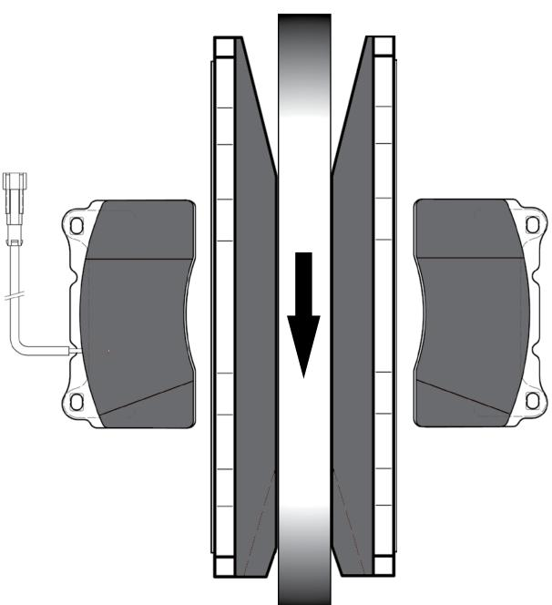
noise. The arrow indicates the disk forward rotation. If the Brake Pads are not fitted as shown above, noise will occur. To ensure the correct fitment in future TRW will print indicator arrows on the back plate.
