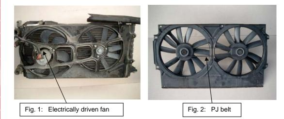
In case additional cooling is needed (cars with air conditioning, with a factory installed tow bar, for taxis, etc), a second fan is installed, in order to pull more cooling air through the radiator. This second fan is then often driven from the first by a 2 or 3 rib PJ belt.
