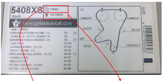
install belt 5408XS, you will need Timing Tool Kit GAT4620, To correctly and in Technical Bulletin # 001 (TB001) you can find tips and points of attention regarding the installation procedure for this drive system.
