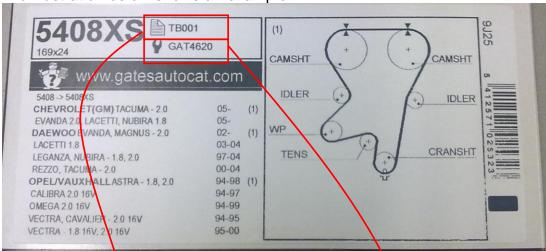
To correctly install belt 5408XS, you will need Timing Tool Kit GAT4620, and in Technical Bulletin # 001 (TB001) you can find tips and points of attention regarding the installation procedure for this drive system.
