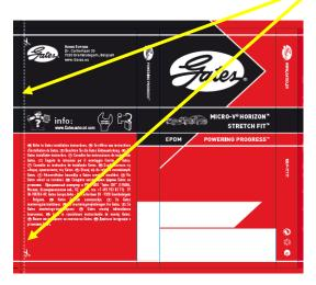
The correct SFT (Stretch Fit<sup>™</sup> tool) can be found on the back of the sleeve (generation Horizon) on the front of the sleeve on the previous generation. The inside sleeve installation procedure repeats also the correct tool to be used for this application.
