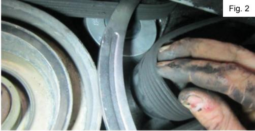
The Gates tensioner must be held in the withdrawn position, by means of an appropriate 15mm wrench, in order to fit the belt (Fig. 2). Gently ease the tensioner on to the belt.
