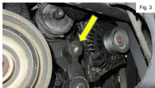
Fitting tip: Remove the (top) idler before taking the old tensioner off (Fig. 3).
