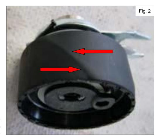
When replacing the timing belt, ensure that a new "ridged" tensioner is installed at the same time.
