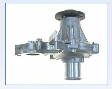
Side profile of the replacement SEM type pump with the front and rear casings pre-assembled.
