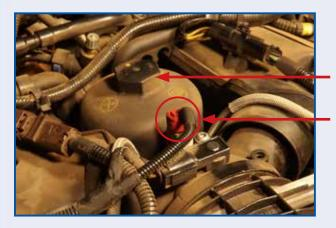
On removal of the engine cover, you will find the oil filter element housing in the centre of the engine at the top.
