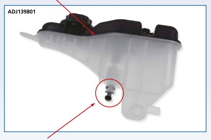
On replacement of the expansion tank, top up with the correct coolant and check for leaks from the coolant hoses after refitting and ensure you connect the level sensor.
