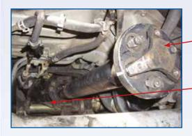
**Driveshaft Coupling (engine side)**
