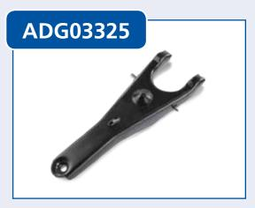
We have found that the cause of the problem can lie with a crack in the clutch release fork, as the release fork on this model can fracture and flex during operation and not allow the clutch to fully disengage.
