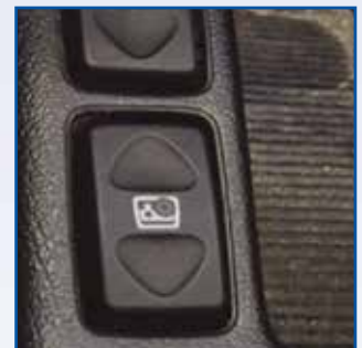
The tailgate window switch is located in the centre console near the handbrake.
