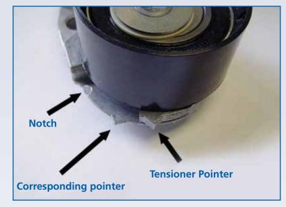
Do not insert any tool into the tensioner assembly to either hold or adjust the tensioner pulley at any point. By doing so could result in the premature failure of the tensioner assembly and any such warranty claims will be rejected.
