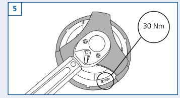
Tighten the fastening ring to 30Nm, then refit the housing to the vehicle and reconnect all fuel pipes and electrical connectors. Start the engine and check for leaks.
