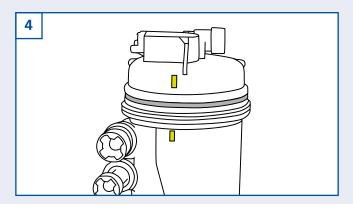
Replace the rubber seal between the two sections of the housing with the one supplied with the new filter. Refit the upper section to the housing by aligning the yellow/green markers.
