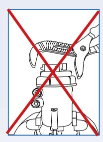
Clamping the plastic housing in a vice and attempting to loosen the filter fastening ring with a large pair of metal-jawed grips is highly likely to result in damage.
