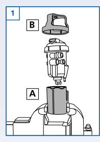
Clamp part 'A' into a vice. Remove fuel filter housing from vehicle, taking care to remove all pipes and all electrical connectors. Place the filter housing into part 'A' and locate part 'B' onto the top of the housing, aligning the six slots of the tool with the filter housing fastening ring.
