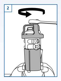
Using a ½" drive ratchet simply undo the fastening ring by turning part 'B' anti-clockwise.
