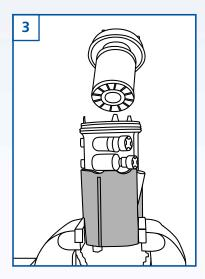
Extract the upper section of the filter housing and replace the fuel filter element (**ADK82327**) taking care not to touch the filter paper on the new element.
