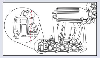
Once removed from the car, hold or carefully clamp the plastic inlet manifold. Mark the coolant blanking section of the manifold that you are about to saw through, making sure that you mark a section slightly larger than the size of the new blanking plate. This is to ensure there is no interference between the manifold and new blanking plate when they are fitted to the engine. Measure twice – cut once!
