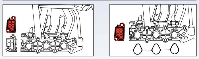
Ensure that the mating surface of the cylinder head is clean and refit the manifold using the new manifold gasket supplied. Fit the new blanking plate onto the cylinder head, using a little RTV if required. Tighten all manifold nuts to the manufacturer's specifications. (15-19Nm)
