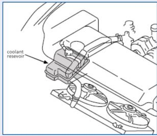
**Note:** Care is required when removing the coolant hose shown in the picture below, in order to avoid damage to the outlet on the radiator.
