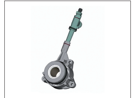
Fig. 2: Concentric slave cylinder with bleed valve in the hydraulic line
