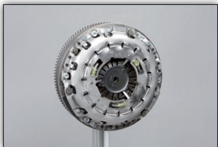
Image 7: Attach the clutch pressure plate and tighten the screws evenly and sequentially using the torque prescribed by the vehicle manufacturer.
