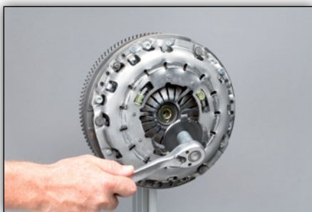
Image 8: Unscrew locking element with appropriate tool and remove. This is no longer required.
