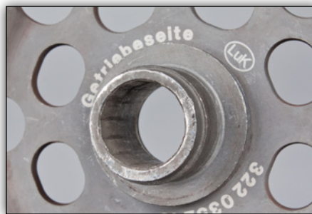
Image 2: Damaged spline profile
