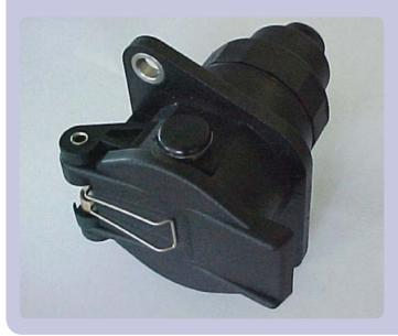
The ISO7638 socket (left) can be fitted to either the motor vehicle or trailer. They are connected by a cable with two male plugs. Alternatively the socket on an articulated motor vehicle can be removed and the cable permanently wired into the vehicle and trailer. In the case of a drawbar trailer, the legislation requires a socket to be fitted.
