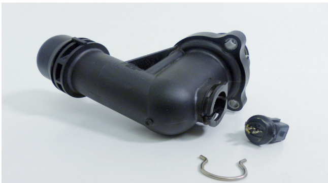
Figure 1: Map-controlled thermostat with retaining clamp released and torn connector.
