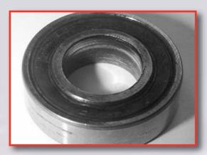
Three flywheel bearings are available from Blue Print: ADC43399 (40mm), ADC43398 (35mm), ADC43397 (32mm)
