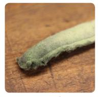
Worn out receiver dryer (or desiccant bag cartridge) often results in clogging of the condenser's inner tube
