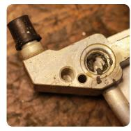
Visible soiling at the condenser inlet
