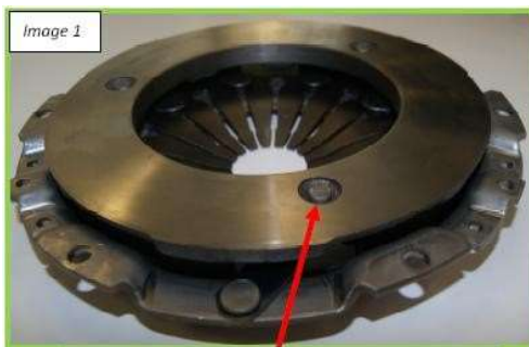
Recessed rivets (below surface area) on pressure plate
