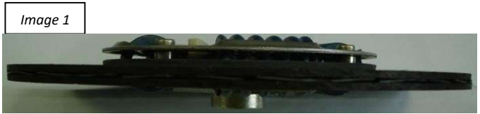
Friction plate side to be mounted flywheel side
