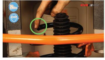
Check overall alignment of assembled unit
