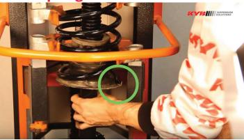
Align top of coil spring with indent in top mount
