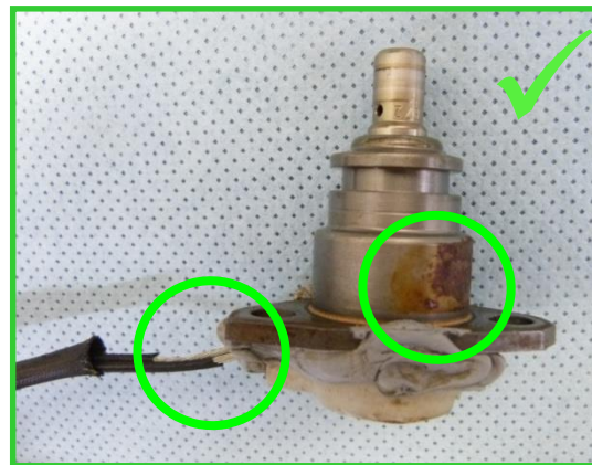
cable / isolation damaged → acceptable corrosion on flange → acceptable
