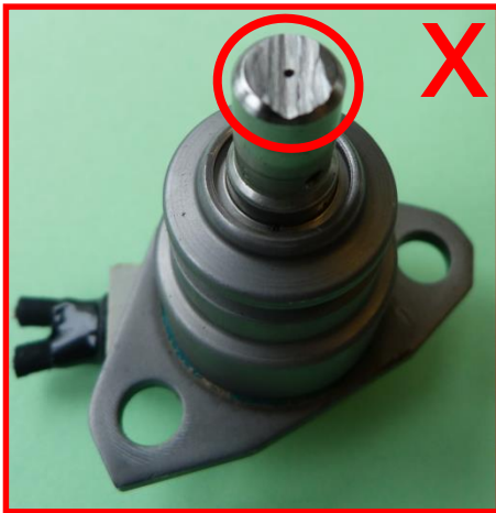
damages on front end of valve unit → not acceptable
