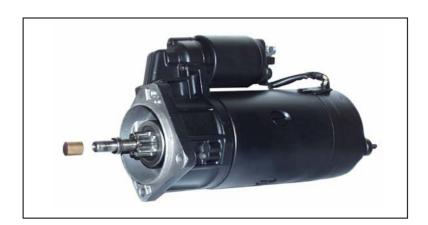
The starter motor is designed with an external shaft support bush which fits in the bell-housing or engine backplate.
