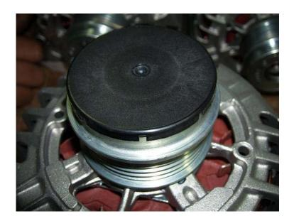
When mounting the unit onto the vehicle make sure the cap remains on the pulley for protection. Its function is to prevent water/dust/debris ingress causing corrosion which seriously affects the lifetime of the clutch pulley.
