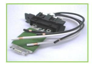
Please note: to eliminate the possibility of making a wiring mistake Valeo Service recommend cutting and crimping only one cable at a time. The loom comes with ready-terminals and crimp connectors, so only one process of crimping and stripping is required.
