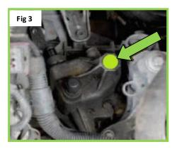
Retro-fitted gearbox with paint mark
