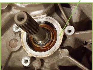
Ensure gearbox mating face is clean and clear of debris
