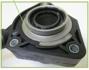
Apply the gasket compound to the CSC back plate
