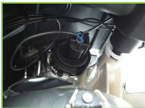
New indicator bulb holder located in the headlight
