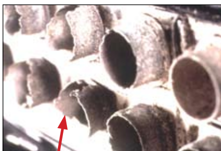
Image 2 Image reveals how corrosion typically attacks the aluminium tubes inside the heater core. When cooling systems are not flushed through thoroughly, or when incorrect / insufficient quantities of antifreeze are used.
