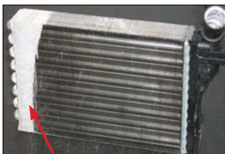
Image 1 Image shows complete heater radiator leaking after nine months of being fitted to the vehicle.
